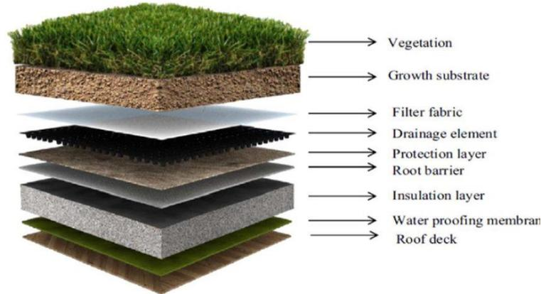
Typical components of a green roof.
